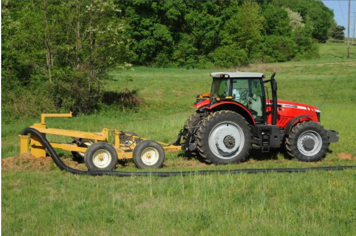
**Model: LWB-6B** Install 5" or 6" tile with the 6" boot kit **\$16,900**
